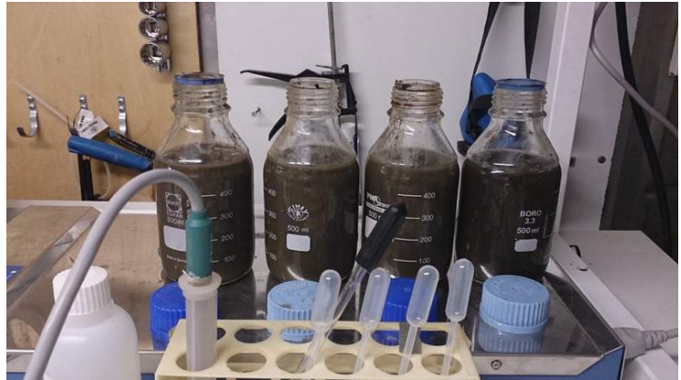
Figure 3 Experimental set-up of acid leaching of algae
