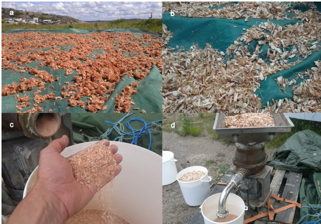
Figure 1 Preparation of dried shrimp shells for use as cadmium adsorbent in leachate. a) Drying of fresh shrimp shells from sea-food industry b) Dry shrimp-shell c) Grinded shrimp-shell (diam. \sim 0,1-3 mm) d) The grinding process using a large kitchen macerator.
