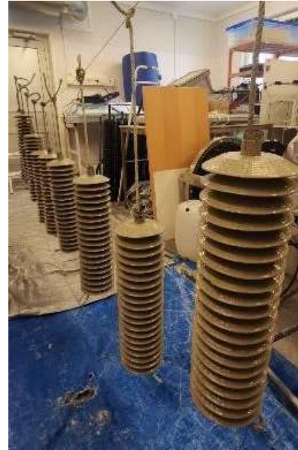
Figure 4. Limed coupelles hung to dry in preparation for deployment. Picture IVL
